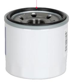
Lubricate the gasket of the new oil filter with a small amount of clean oil. This will ensure that the gasket does not bind when it meets the mating surface on the oil filter housing.
